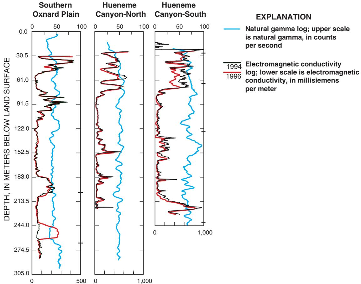
**Fig. 7** Electromagnetic-conductivity borehole logs from three wells in Ventura County, California. Repeated measurement of the conductivity of the aquifer at the three wells indicates that conductivity decreased in the shallower parts of the aquifer during the 2-year interval. (Modified from Hanson et al. 2009)
