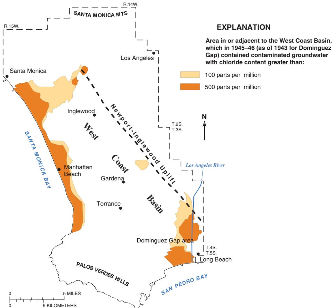
**Fig. 6** Chloride concentrations in coastal Los Angeles (California) in the mid-1940s. (Modified from Poland et al. 1959, plate 16)
