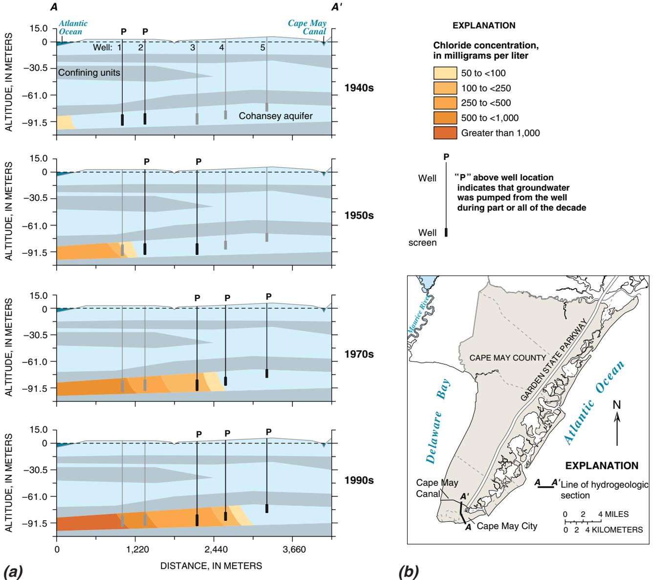
**Fig. 2** a Hydrogeologic sections showing lateral encroachment of saltwater and contamination of supply wells in the Cohanseay aquifer at the Cape May City (New Jersey) well field, 1940s to 1990s. b Map of Cape May County, New Jersey. (Modified from Lacombe and Carleton 2002)
